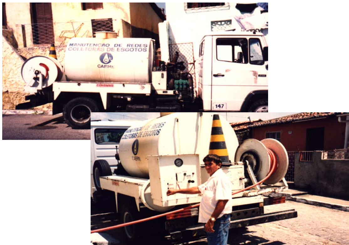
Plate 4.33. The vacuum tanker used by the sewerage maintenance crew of Rocas/Santos Reis
