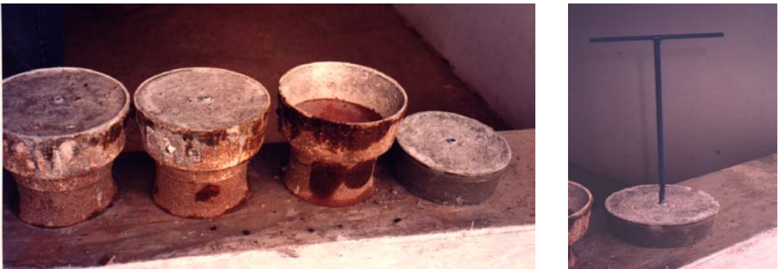
Plates 4.42. The new mould for the mortar weight and the key to lift the covers
