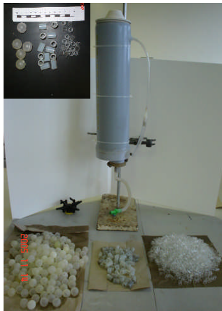
Figure 6.2 Packed column for the ammonia absorption system AS3
