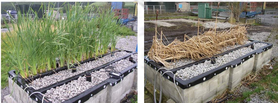
Figure 5.5. The pilot-scale rock filters (bottom, aerated RF; middle, unaerated RF) and subsurface horizontal-flow constructed wetland (top) at Esholt, Bradford. Each unit is 4 \times 0.5 \times 0.5 m.
