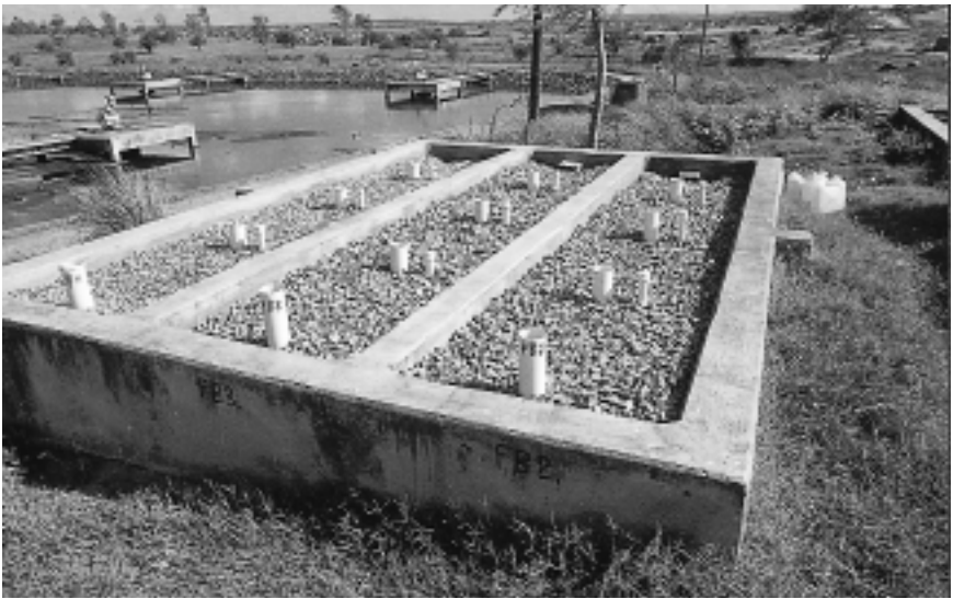
Figure 2.7: Experimental rock filters receiving effluent from the primary maturation pond.
